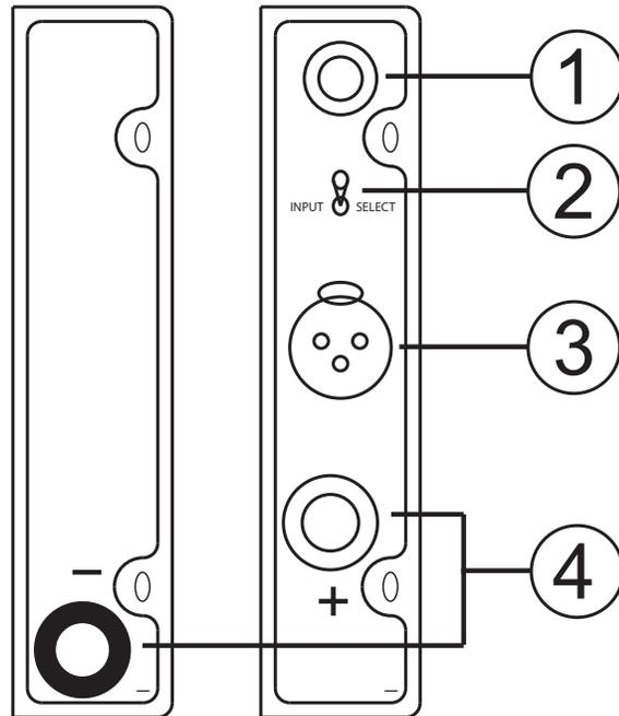
**Note: Each Differential Reference Amplifier channel has a separate Balanced and Unbalanced input and an independent Input Selector switch.**
