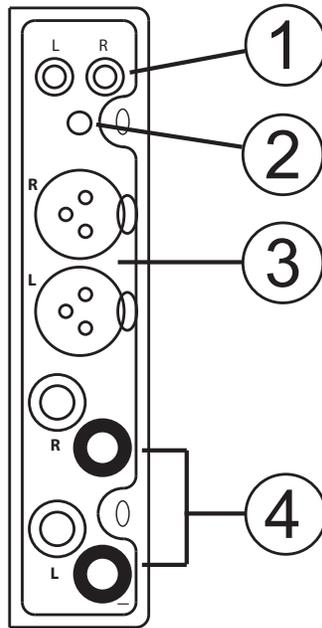
**Note: Each Amplifier Module has separate Balanced and Unbalanced inputs and an independent Input Selector switch.**
