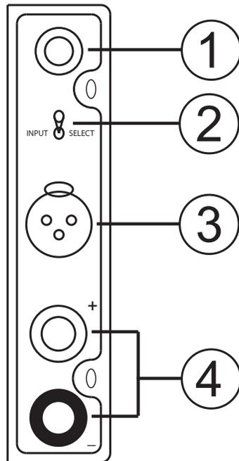
**Note: Each Amplifier Module has a separate Balanced and Unbalanced input and an independent Input Selector switch.**
