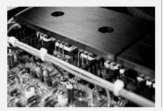
No part of a Naim product escapes the careful scrutiny of our engineers. The position and layout of wires that carry signals and power around a product is very important. Run a delicate audio signal line next to a noisy power line for example, and it will pick up noise and distortion.
