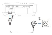
A power supply cord connected to a socketoutlet with protective earthing connection.
