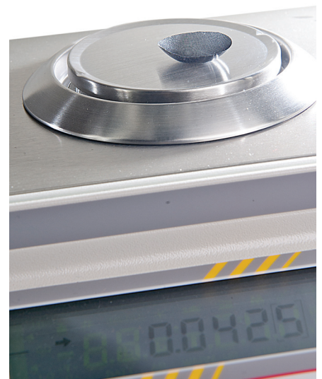
The ZENSOR tweeter is constructed on the basis of an ultra light-weight weave fabric. Compared to most soft dome tweeters in the market the DALI dome material is less than half the weight; 0.056 mg per mm 2 .
