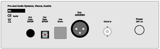
Make all connections whilst the CD player is disconnected from the power supply. Never use any other power supply than the one supplied with the unit, except of Pro-Ject Power Box.
