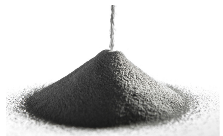
The individually coated magnet granules makes it possible to mold a pole piece that is not electrical conductive.
