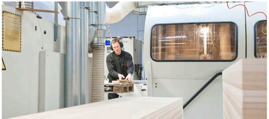
Cutting the MDF boards for OPTICON cabinet production.
