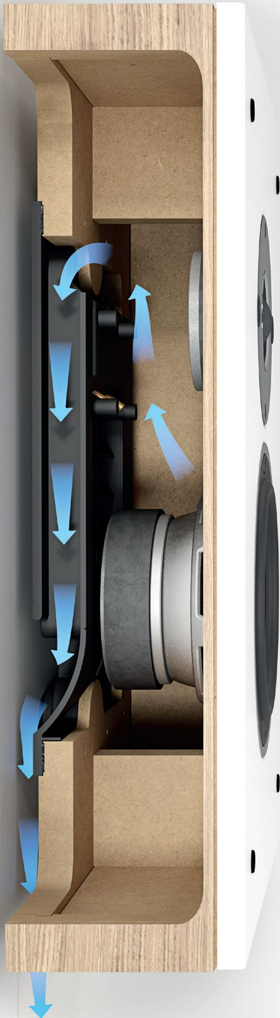
The OBERON ON-WALL takes the use of the rear wall to a whole new level. Using the unique port design originally introduced with our RUBICON LCR, the OBERON ON-WALL bass ports fire downwards, letting the ports and the wall work together to extend the bass reproduction far beyond what should be possible from such a compact cabinet.
