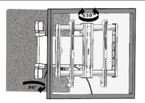
Connect the cables to your TV and route through the cable clips, **Note:** Leave slack in the cables for arm movement.
