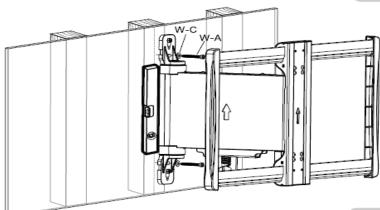
Install the other two screws and level the wall plate, then tighten all screws for security.
