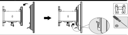
Lift and hook the TV onto the wall mount.
