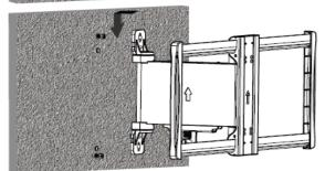
Align the big holes on the wall plate to the screws in the wall and lower the wall plate.
