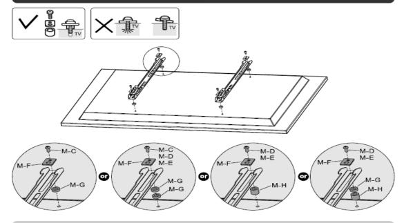
Note: Choose the appropriate screws, washers and spacers (if necessary) according to the type of screen.
