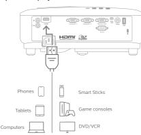
2 If the projector does not automatically switch to the correct input source, press ᢓ on the projector or **Source** on the remote control to switch the input source to *HDMI*.
