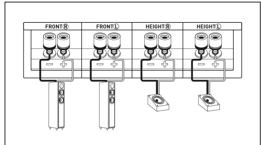
Connect the inputs of your Monitor ATM to the FRONT HEIGHT (or PRESENCE) terminals of your amplifier. Then, connect the MAIN inputs of your Monitor IX to the FRONT (or MAIN) terminals of your amplifier.
