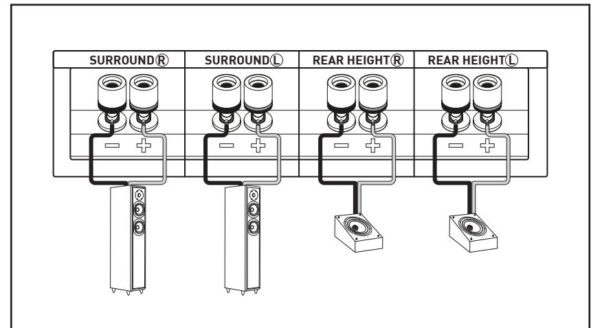
Connect the inputs of your Monitor ATM to the REAR HEIGHT (or PRESENCE) terminals of your amplifier. Then, connect the MAIN inputs of your Monitor IX to the SURROUND terminals of your amplifier.
