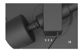
Slip the loop of the anti-skating weight's thread over the third groove of the stub to set the correct anti-skating force for the factory-fitted cartridge. Feed the thread through the loop of the wire support (17).
