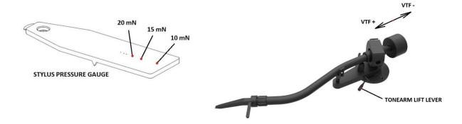
To adjust the amount of pressure, carefully move the counterweight (6) along the support rod, until the stylus pressure is sufficient to raise the pressure gauge to the level position. Moving the counterweight (6) away from the cartridge will reduce pressure and towards will increase pressure.
