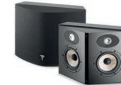
Aria SR900 is a 2-way bipolar surround loudspeaker with the same acoustic characteristics as the other loudspeakers in the Aria range. Composed of two 5" (13cm) woofers with Flax sandwich cones, it provides very high-definition and natural sound. For the treble register, there are two aluminum/magnesium inverted dome tweeters with Poron suspension and a waveguide for a better control of directivity.
