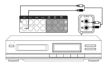
**Recording connections** Connect the REC OUT terminals to the input (LINE IN) terminals on the tape deck using the pin-plug cord.
