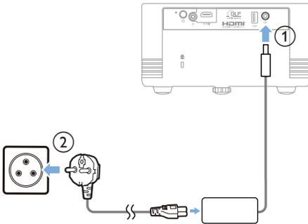
A power supply cord connected to a socket-outlet with protective earthing connection.
