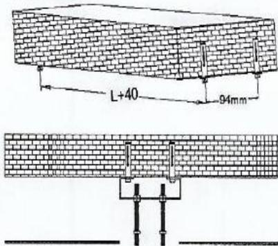
Distance de fixation: L+40mm x 94 mm
