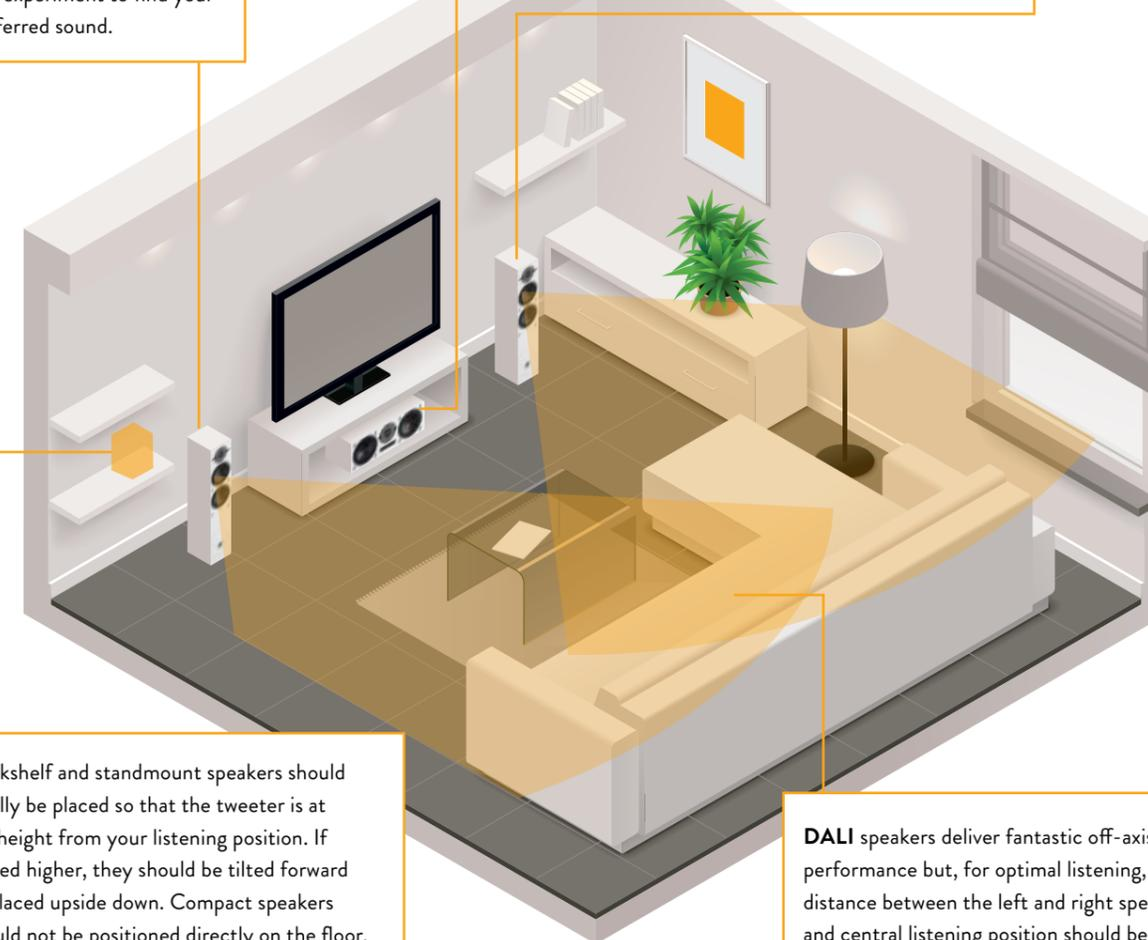
Bookshelf and standmount speakers should ideally be placed so that the tweeter is at ear height from your listening position. If placed higher, they should be tilted forward or placed upside down. Compact speakers should not be positioned directly on the floor.
