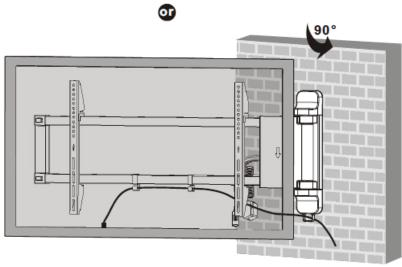
Connect the cables to your TV and route through the cable clips. **Note:** Leave slack in the cables for arm movement.
