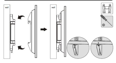
Tighten the bottom bolts to secure the adapter brackets to the wall mount.
