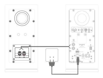
Connect the RED(+) and BLACK(-) terminals from the left speaker to the corresponding terminals on the right speaker using the included speaker cable. Insulation on cable must be stripped on all ends.
