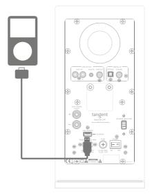
In case of low battery of your device, you can charge it on the USB plug at the back of your Spectrum X5BT.
