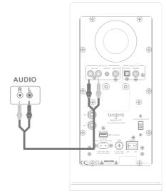
Connect any audio analog stereo source with RCA cable.
