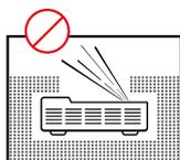
The Laser TV must not be set up in an enclosed space with limited ventilation. Doing so would cause the device to overheat.
