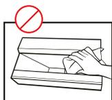
The lens must not be touched directly or wiped with a cleaning cloth. Doing so may damage the lens coating, which would negatively affect the image quality.
